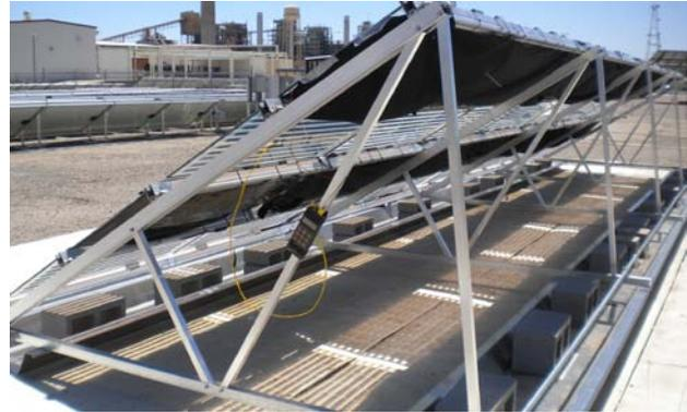
**Figure 6. Shading experiment covering back of module with black canvas that blocks all albedo and diffuse light that would otherwise be accepted by bifacial modules.**
