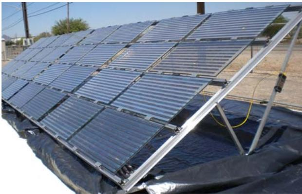
**Figure 5. Shading experiment covering mock white roof with black plastic that reflects light onto backside of modules.**
